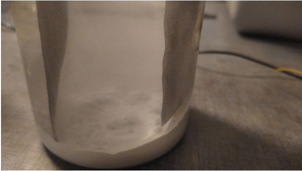
Figure 2: pre process: The electrode which hangs on the spring scale is plunged and immersed by the electrolyte. The white powder at the ground is precipitated zinc oxide (ZnO).
