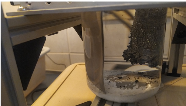
Figure 3: post process: the regenerated zinc was accumulated as a sponge on the right electrode. The white zinc oxide powder has been gone.
