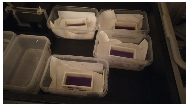
Figure 11: The boxes were placed into a bigger containment (with a lid) and then left for 10 weeks
