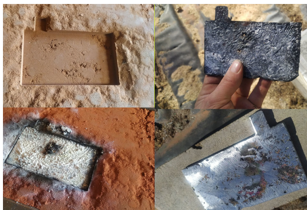
Figure 13: Producing a thicker zinc anode by casting
