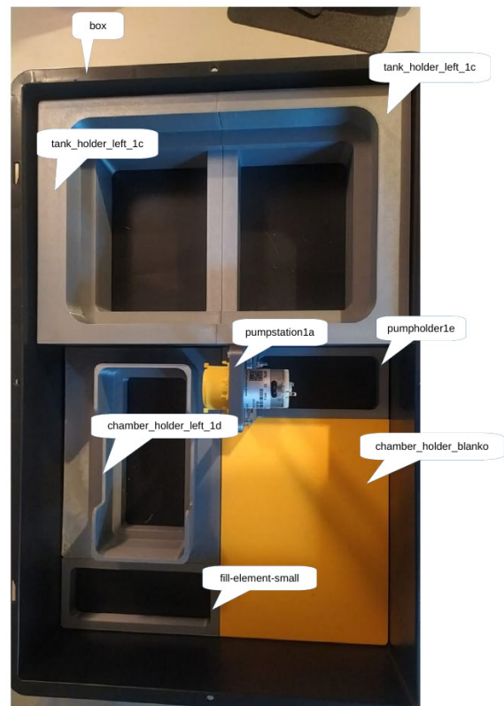
Figure 6: Survey of the containing box with structural elements, mostly 3d-printed
