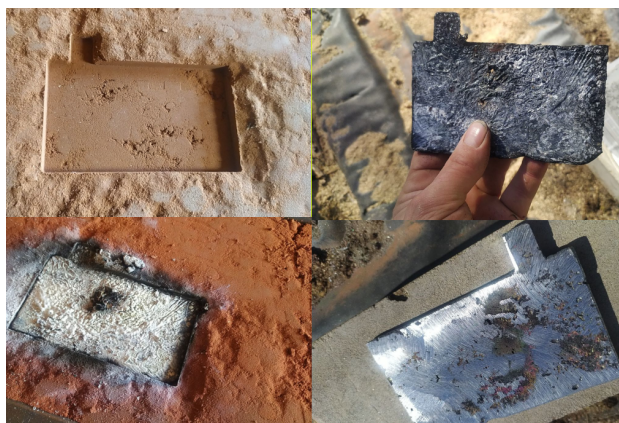
Figure 13: Producing a thicker zinc anode by casting
