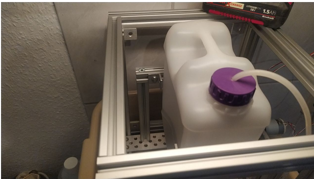
Figure 3: The pump pulls the electrolyte out of the cell's outlet and let it drip from above into the buffer-reservoir
